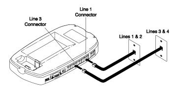
Connecting the AirWay 516 Controller to 2-line wall jacks
