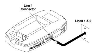
Connecting the AirWay 308 Controller to 2-line wall jacks
