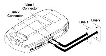
Connecting the AirWay 308 Controller to single-line wall jacks
