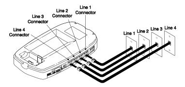
Connecting the AirWay 516 Controller to single-line wall jacks
